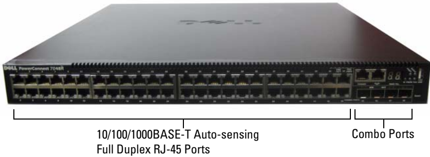
Figure 1-6. PowerConnect 7048R with 48 10/100/1000BASE-T Ports
